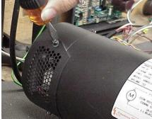
Locate the brush and the clip holding it in place. On one side of the motor, the clip will be under the brush, and on the other side it will be on top of the brush.
