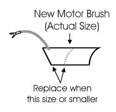
After inspecting the brushes, place the brush and clip back into place. The clip will "click" into its resting position. Reattach the vent flaps that cover the motor brushes.
